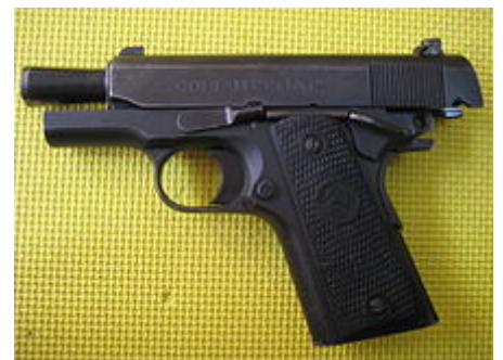
A Colt M1991A1 Compact ORM pistol with slide locked back to expose bull barrel.
