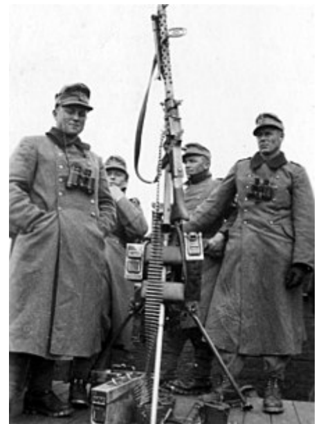
Tripod mounted MG 34 setup for its anti-aircraft role
