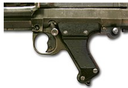
MG 34 double-crescent trigger, E= "einzelfeuer," semi-automatic fire, D= "dauerfeuer," full automatic fire
