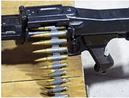
MG 34 with inserted Gurt 34 reusable non-disintegrating metal ammunition belt
